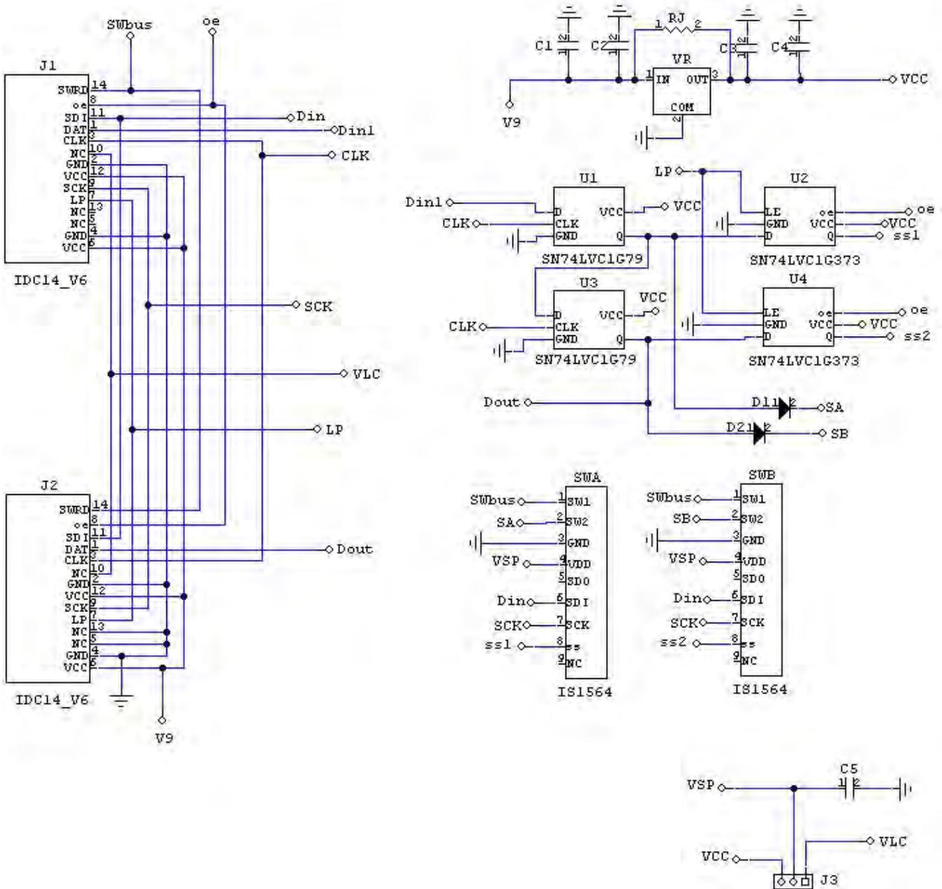
**Logic Board Schematic for Two LCD 64x32 RGB SmartDisplays (IS-L02F1-C)**
