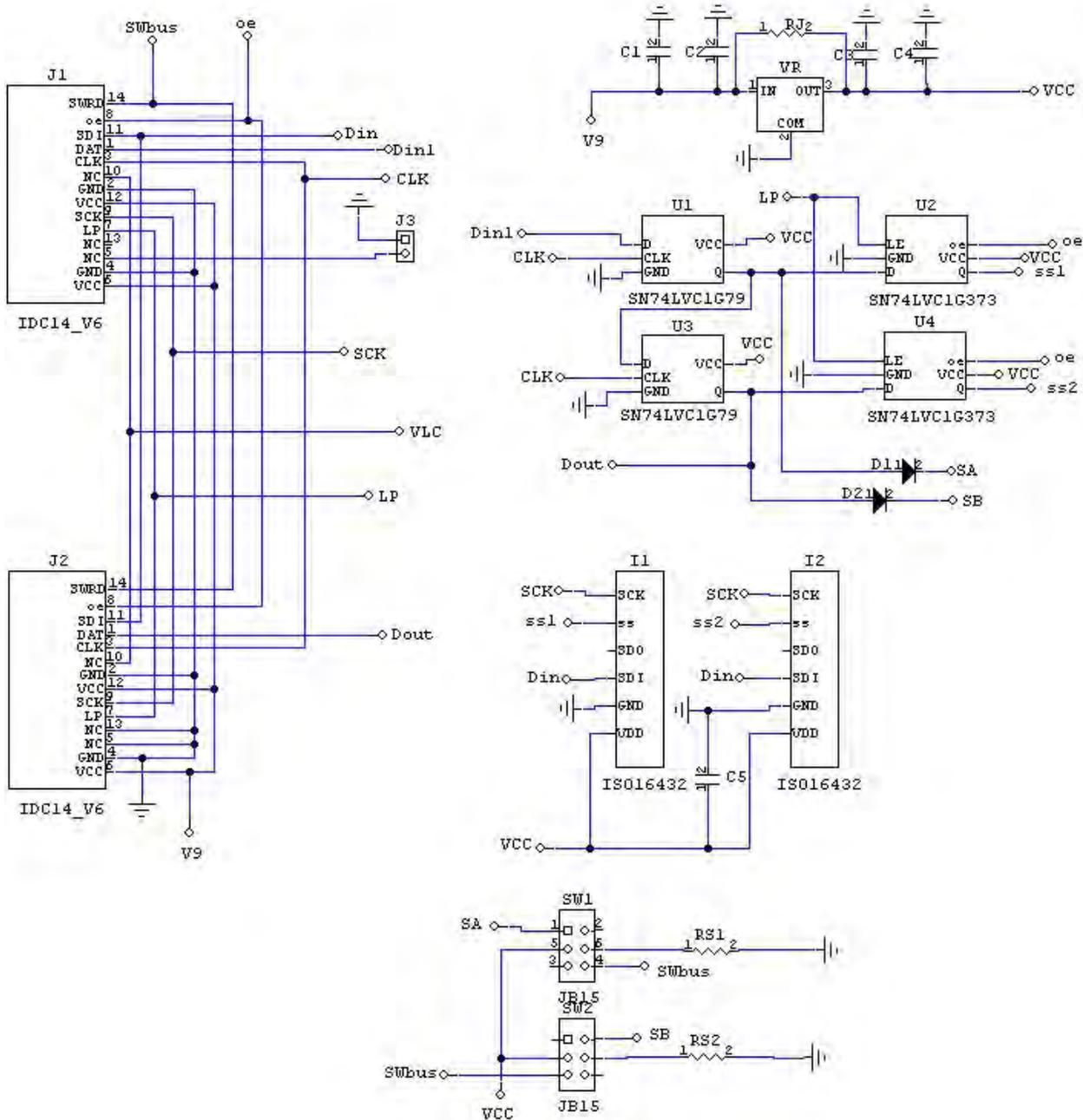
**Logic Board Schematic for Two LCD 64x32 RGB Compact SmartSwitches (IS-L02H2-C)**
